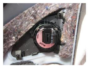
The stock tweeters use an inline capacitor to filter the high frequencies on the tweeter itself, so you can use the stock wiring to feed your new tweeters, just ensure you install whatever filter is supplied with them. Components with an inline filter are far easier to install than ones with a full on crossover unit.
