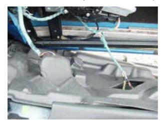
Then the door card is free. Place face down on a soft surface and remove the wiring and then the main speaker, 3 Torx screws.
