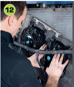
The next task is to cooling fans at the top of the radiator pack. The fans are secured with radiator ties that are fed through the radiator fins from the rear and then secured. Regal opted to temporarily radiator mounting bolts and move it forward, allowing the ties to be fed through it alone. You can feed them through both the cooling and air con radiators if you want to.
