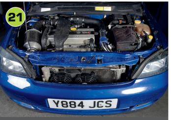
Refit the front bumper, remembering to reconnect the wiring for the foglights and outside temperature sensor. Replace the push down rivets along the top of the bumper and the bottom at the subframe. Refit the Torx bolts at the edges, ensuring the bumper is located in the runners at the leading edge of the front wings correctly and the panel gaps are nice and even.
