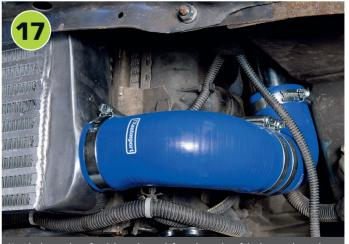
Next is the section of stainless pipework from the outlet of the intercooler to the engine bay. Again, follow the diagram supplied and use a reducer section on the outlet of the intercooler. Feed the pipework up behind the radiator and into the engine bay. Ensure the mounting section for the boost sensor is in the correct location. Refit the boost sensor and multiplug. Tighten all jubilee clips.
