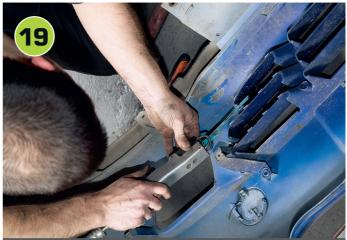
Trial-fit the front bumper. Cars with GSi front bumpers shouldn't need any modification, however the Coupe bumper requires small sections of plastic removed from the rear to enable it to clear the intercooler. Regal used an air powered hacksaw to cut back small sections of the plastic grille but sharp snips will do. Cut small sections at a time, trial-fitting the bumper until it clears fully.
