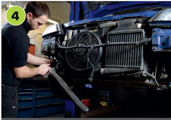
Remove the standard rubber boost hoses. One runs from the turbo outlet to the base of the intercooler and the other runs from the intercooler to the top hat at the rear of the engine. All are secured by jubilee clips. Also remove the boost sensor located at the top of the intercooler by removing the T25 Torx bolt and the multiplug. Put the sensor somewhere safe, you'll need it again.
