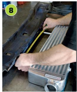
The mounts on the top of the intercooler are 350 mm apart, so either side of your crash bar and again mark the points. Offer the intercooler up to the crash bar. ensuring the lines you have marked correspond directly to the mounts on top of the always the case, measure twice and satisfied, move the intercooler safely out of the way.
