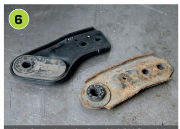
In this case Regal opted to move the radiator pack back slightly. The standard brackets (bottom) were swapped for Astra VXR items with the rubber locating section turned round, which moves the radiator pack backwards by approximately 20 mm. The top locating brackets were spaced back using additional nuts, again to aid clearance. This isn't always strictly necessary but does help in later stages.
