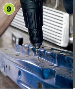
Drill two small pilot holes in the top edge of the crash bar, approximately its leading edge. Again offer up the intercooler to ensure the holes correspond to the mounting points on the intercooler. Assuming they do, enlarge the pilot holes using a 13 mm drill bit. Clean up any rough edges and if attention to detail is your thing, apply a small amount of paint to the exposed bare metal.
