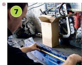
Next task is to TX Autosport intercooler. The intercooler mounts to the existing crash fitting kit supplied with the intercooler. Lay a bench or the floor with the top surface facing upwards, i.e. as fitted to the car. Find the centre of mark it using predrilled holes as a reference point.
