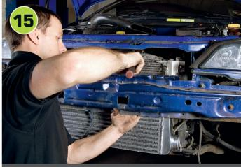
Refit the crash bar and intercooler assembly, ensuring there is sufficient clearance and the wiring is not trapped or pulled excessively tight. If required, reposition the intercooler and/or fans until there is clearance. Ensure the section of loom for the outside temperature sensor is fed between the crash bar and intercooler. If all is well, firmly tighten the bolts that mount the intercooler to the crash bar.
