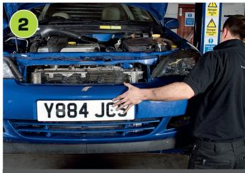
Pull the bumper towards you slightly and then reach down and disconnect the fog light multiplugs and also the multiplug for the outside temperature sensor. Remove the bumper completely, taking care not to drop it face down. Store it safely out of the way on piece of cardboard. Put all the bolts and fittings somewhere safe, a small box or magnetic tray is perfect... the floor isn't.
