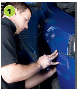
easier, raise the front off the ground. Car ramps or axle stands are fine but just make wheels are choked and you're on firm level ground. Remove the small Torx bolts that secure the bumper just in front of the wheels, remove the push down rivets along its top edge at the grille and finally the push down rivets underneath that secure it to the subframe.
