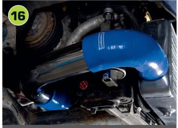
The first section of stainless pipe runs from the turbo outlet to the intercooler inlet. Following the supplied diagram, assemble the pipework using the silicone joining sections. Don't tighten the jubilee clips until the pipework is in place and any adjustments have been made.
