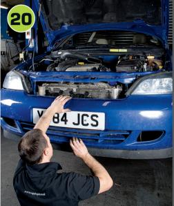
Before refitting the bumper, recheck every nut, bolt and jubilee clip, ensuring they have all been refitted correctly and are sufficiently tight. Ensure the jubilee clips have been seated correctly and evenly on the silicone hoses. Check all wiring is safely secured with especially the section of loom that crash bar, making trapped or pulled excessively tight.
