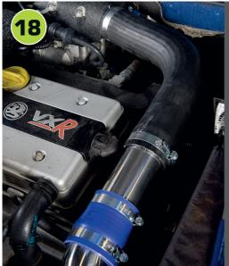
The intercooler pipework is designed to connect to the existing top hose, however you will need to cut the original hose halfway and fit it over the new stainless pipework. If you have a TX Autosport top hat kit or an alternative hard pipe you will need to connect these to the intercooler pipework. As ours pipe, this is what the images.
