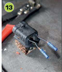
If you have opted to move the air con radiator forward, refit it back in place and refit the bolts. The next step is to hardwire the twin fans to the original wiring loom. Cut the multiplug from the original fan assembly. You can either solder the wiring or alternatively use Either way, ensure properly insulated and ideally sealed using heatshrink or insulating tape.
