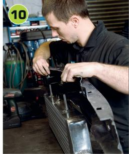
Using the supplied fitting kit, bolt the the inside of the crash bar so they extend backwards towards the engine bay. Next, bolt the intercooler to the box section mounts using the bolts supplied. Do not overtighten these, finger tight is sufficient for the time being. The intercooler is symmetrical so it won't matter which mounted.
