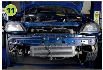
Refit the crash bar and intercooler combo to the car, ensuring it is fully located on its mounts. You may need to use a soft faced hammer or refit the bolts to make sure it is correctly seated. Once seated, double check the intercooler is fitted centrally on the crash bar and that it is clearing the original components and bodywork. Remove the crash bar once more and place safely out of the way.
