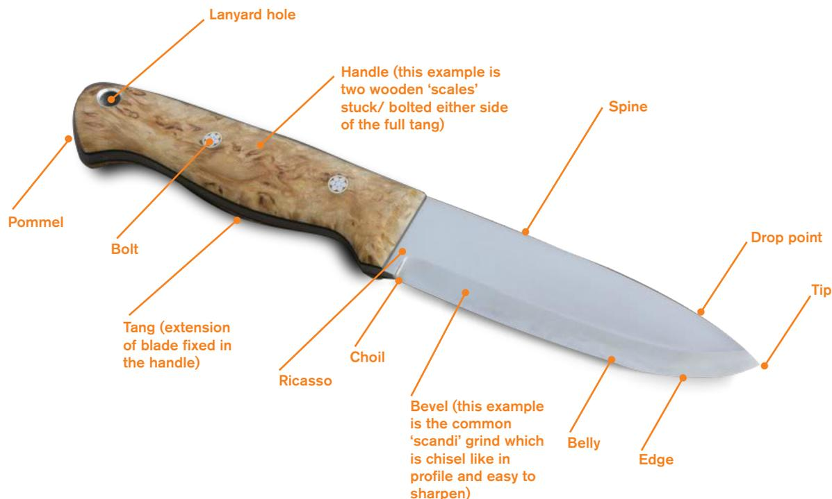
A large fixed blade can be used to whittle away larger sections of material to give a rough shape. It is not good for fine detail as there is less control over the blade. A large fixed blade can also be used for splitting wood.
