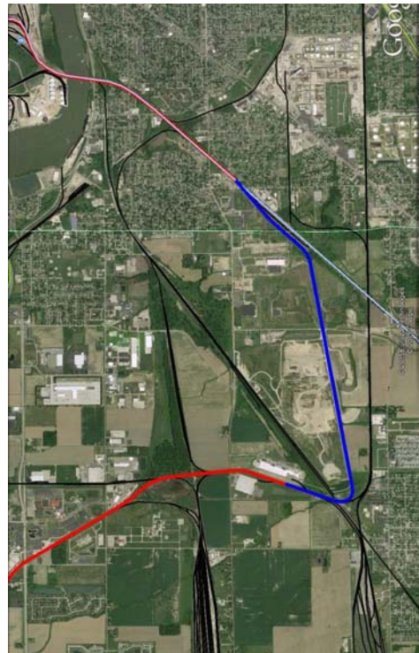
Illustration 8: On Toledo's southeast side, from Walbridge north to East Toledo, CSX's 2.75-mile Stanley Secondary (dark-blue line) links CSX's Toledo Branch Sub-division (red line) from Bowling Green to NS's Chicago Line (red/light-blue line) to Toledo's MLK Plaza station at the upper-left of the satellite image. The Stanley Secondary is need of track and signal improvements prior to the introduction of passenger service.
