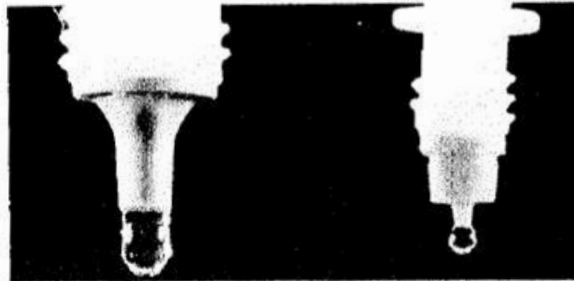
Fig. 2 (Brown, Hotchkiss, and Davis). A standard-sized eyedrop (left) from a commercial eyedropper tip compared to a smaller eyedrop produced by one of the smaller tips we used (outer diameter = 0.047 inch; inner diameter = 0.020 inch).
