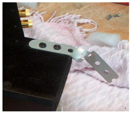
To get the best performance from the sub it is vital that it is secured well to the chassis of the car. It is advisable to install the 2nd bracket supplied at the rear of the sub. You can do this with the sub insitu, screw the bracket to the top of the sub and then bolt to the flange on the wheelarch as shown. This gives the sub rock hard stability which will allow it to perform at its best.
