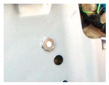
Now you need to cut off the unnecessary flanges on the rear wing seam using a hacksaw, shown below already removed. These are the tabs that stand proud of the seam and were used to secure the wiring loom, and will foul on the bottom of the AMSS.
