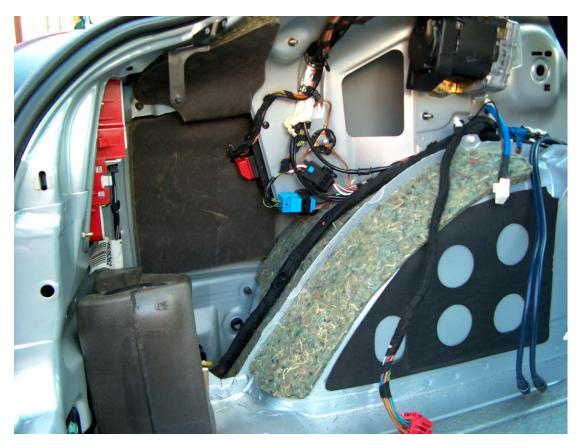
The AMSS is slightly larger than the original so some of the obstacles in the rear wing need to be tidied up before the unit will fit properly.
