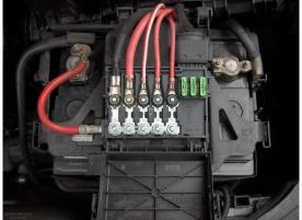
Make sure you take the inline fuse out before connecting the remainder of the cable it to the battery.
