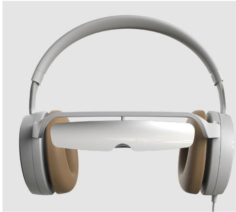
1. Pico Interactive's Eagle headset features over-ear, noise-cancelling headphones and a removable high-definition OLED display band.
