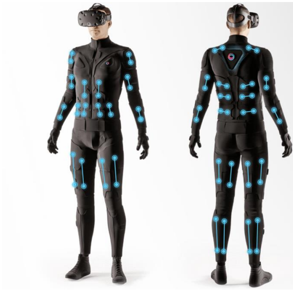
5. The Teslasuit incorporates 46 haptic points that can provide different feedback to the wearer, such as weight simulation.
