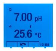
In the above case 2 sensors have been selected in the menu format-selection. Further the sensors 2 + 4 have been chosen in the menu display mode. The upward arrow shows a control of the temperature upwards, that means the heating is active at this moment.
