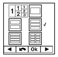
In this menu you can adjust how many metered values shall be displayed simultaneously. The possibility to display 1, 2, 3, 4 or 8 sensosors at a time is at your disposal. In order to select use the keys or to jump to the desired format and confirm it with the key **Ok**. Then a papers behind the desired format. In order to save the settings press the key. Now you are in the main menu again.
