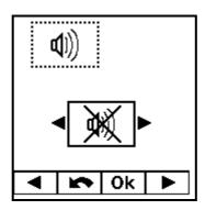
In this menu the key-tone <u>and</u> the acoustic alarm are activated/deactivated. For adjusting use the keys **d** or **b**. In order to save the settings press the key **Ok**. Now you are in the main menu again.
