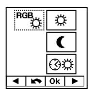
The RGB menu has three submenus. In case of the first two, colors and brightness of the background lighting for day and night are adjusted according to the symbols. As soon as you get into one of these menus, the controller for the red colour (R) is active. For adjusting the colours use the keys
