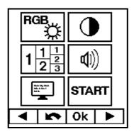
From this menu on you get to the submenus. The selected submenu is displayed invertedly. By the keys and you can jump to the differnet menu items. With the **Ok** key you will then get into the respective submenu. For getting back to the main menu press the key.
