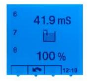
Here, the display for 3 sensors has been selected in the menu format-selection. Further the sensors 6 + 7 + 8 have been selected for being displayed in the menu display-mode.
