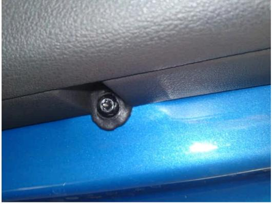
**Step 3:**You now need to start to unclip the **card** from the **door** starting at the bottom
