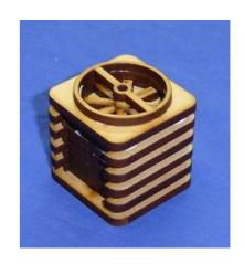
6. Glue the **Control Panel** to the indented section of the stacked **Heat Sink Plates**, taking note to have the two holes in the **Control Panel** uppermost as shown.
