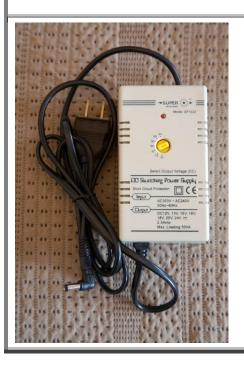
For testing purposes I used a variable voltage power pack.
