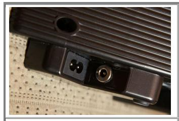
I placed the DC power jack next to the power socket.
