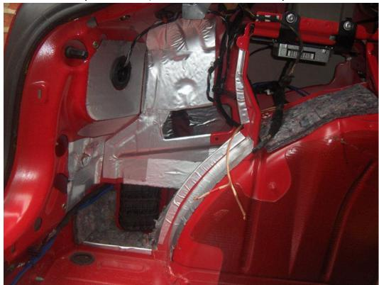
Before fitting the AMSS enclosure you'll want to run the RCA adapter loom from the top of the Bose amp behind the drivers side boot panel, underneath the boot sill (the blue cable shown above & below) and round the back of the sub to the amp (depending on amp location). Fish it behind the inner panel and up to the top of the wheelarch so it won't foul the enclosure.
