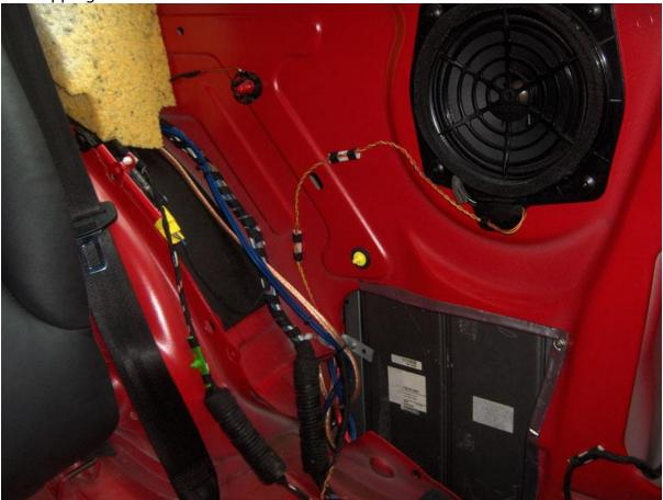
With the amp firmly in position test everything still works correctly before the rear speaker panel is refitted. Zip tie all new cabling securely before refitting the panels.
