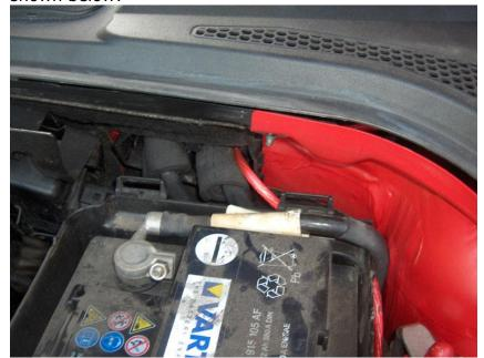
Then along and up to the fuse panel beside the battery. If you bought my install kit then I included two nuts and a VAG 40amp fuse, so there is no need to mount a separate fuse, just bolt the fuse and the cable as shown below (BUT DON'T DO IT YET!). Leave the fuse out until you have completed wiring the up the amp. If you are
