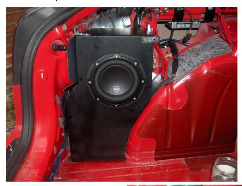
With the brackets tightened the sub should be rock solid, you should be able to rock the car by rocking the sub enclosure. This is vital for it to perform properly. If it's wobbly then it is not correctly fitted.
