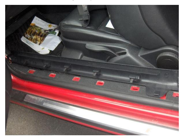
Now for the rear speaker panel. Remove the rear seat base by pushing it towards the rear of the car and lifting, they can be really stubborn. It's hooked at the back as well, same process. Fold down the passenger side seat back. Starting at the base of the door pillar, pull the panel free, working your way up to the top of the panel. The panel is held on with metal clips and plastic poppers,
