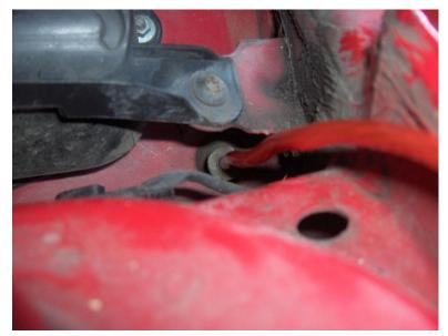
This enters the cabin down the side of the glovebox. Cut off the end of the nipple on the grommet (I use a pair of end cutters) and poke a wire coathanger through. When you've located the other end in the footwell, tape the power cable to it and pull it through from the engine side. Be careful as the grommet can get pulled out, use some fairy liquid to ease it through.
