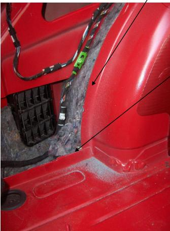
At the bottom of the wheelarch trim off the bottom seam so that it forms a right angle with the wheelarch seam.
