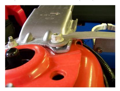
I thought about my getting out my cutting tools and notching out the brace but rejected that idea in about 10 seconds. I finally decided to try sandwiching the bracket between the brace and the shock tower. I used a pair of external star
