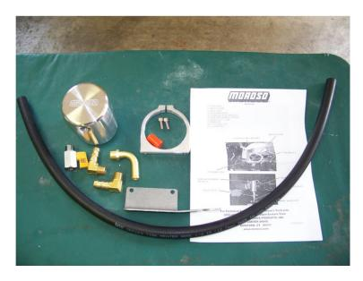
My only disappointment with the parts was the hose was clearly marked "Heater Hose". While I don't expect tons of oil to be flowing through it (there better not!), for \$140 you think they could at least provide hose rated for fuel and oil exposure. That's as bad as putting a cheap Chinese transmission in an otherwise world class performance car.
