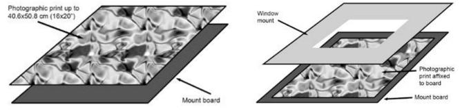
Option 1: Flush mounted on single board
