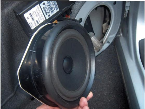
If you are Dynamatting the inner skin then do this with the speaker out so the sound deadening goes under the adapter when fitted
