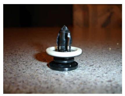
You now need to start to unclip the **card** from the **door** starting at the bottom and working around. They're very tight at first and you seem to have to pull very hard but they do come off! I started at the bottom by the speaker.
