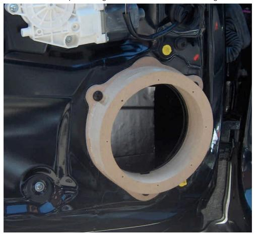
Mount the new components to the adapter.
