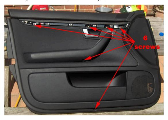
Remove the 6 screws Lower the window
