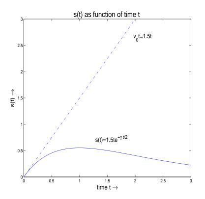
FIG. 4: 1.9(a) Plot of s(t) in the critically damped system
