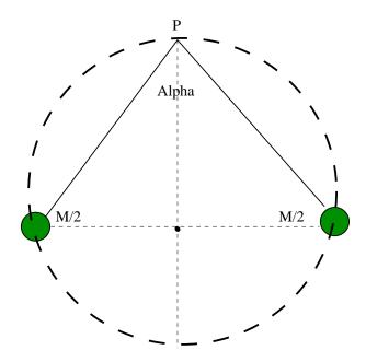
FIG. 3: 1.8 Simple Two Mass Pendulum
