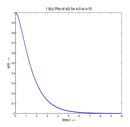
FIG. 5: 1.9(c) Plot of s(t) in the overdamped system
