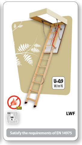
The **LWF folding** 3 section Fire-Resistant Loft Ladder thanks to its high fire-resistant properties, **El<sub>2</sub>: 30 min** (**according to EN 13501-2**) is perfect for installations subject to stipulations as specified in the building regulations.
