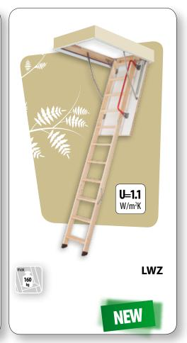
The **LWZ** is 3-section folding wooden ladders with an insulated hatch. The hatch box consists of metal frame integrated with wooden box. The steel frame integrated with finishing lining slats and the system of quick installation; both simplify installation and reduce the time of setting the ladders in the ceiling.
