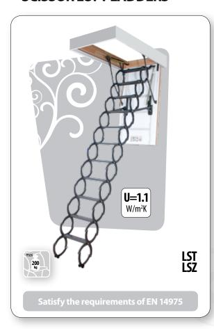
The **LST** loft ladder (wooden box with finishing slats), the **LSZ** (metal frame with finishing slats, integrated with a wooden box) are scissors loft ladders with a white insluated hatch. The scissors ladder construction helps the folded ladder to take less space allowing the ladder to be installed in smaller openings (the smallest ladder size is 50 x 80 cm).
