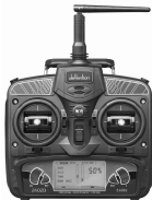
3. Pull down the throttle stick and throttle trim of transmitter to the lowest position, and then move the elevator trim, aileron trim, and rudder trim at the neutral positions, respectively.
