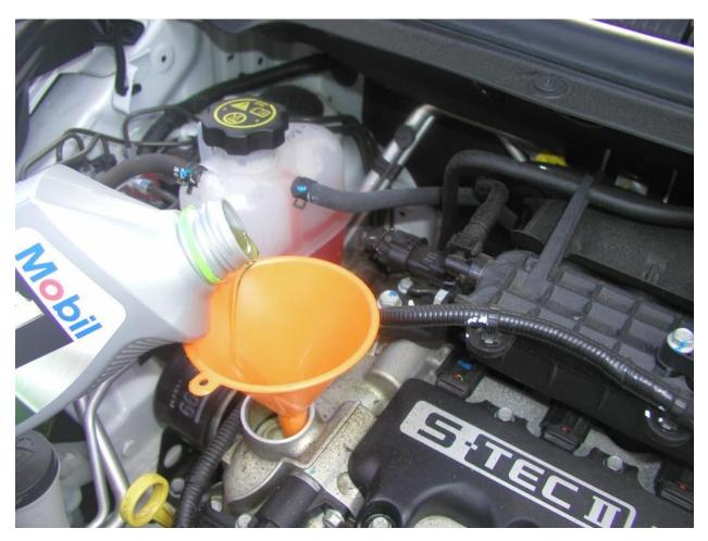
Loosen the oil fill cap and add 4 quarts of motor oil to the crankcase. Check with the dipstick that the oil is at the right level. It should be between the dots on the dipstick which indicate the minimum and maximum level.
