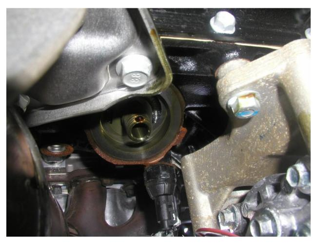
The above picture shows the oil filter removed. Note that the surface should be clean and free of any gasket material. When installing the new filter, make sure that it is threaded properly.
