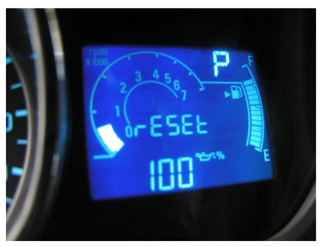
Last, the Oil Life Monitor needs to be reset. This is important for your personal records and also for OnStar to recognize that an oil change has been performed.
