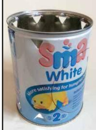
**2.** Using the can piercer, make holes around the top of the tin and around the bottom. IMPORTANT: Don't make any holes too close to where you have marked out the circle.
