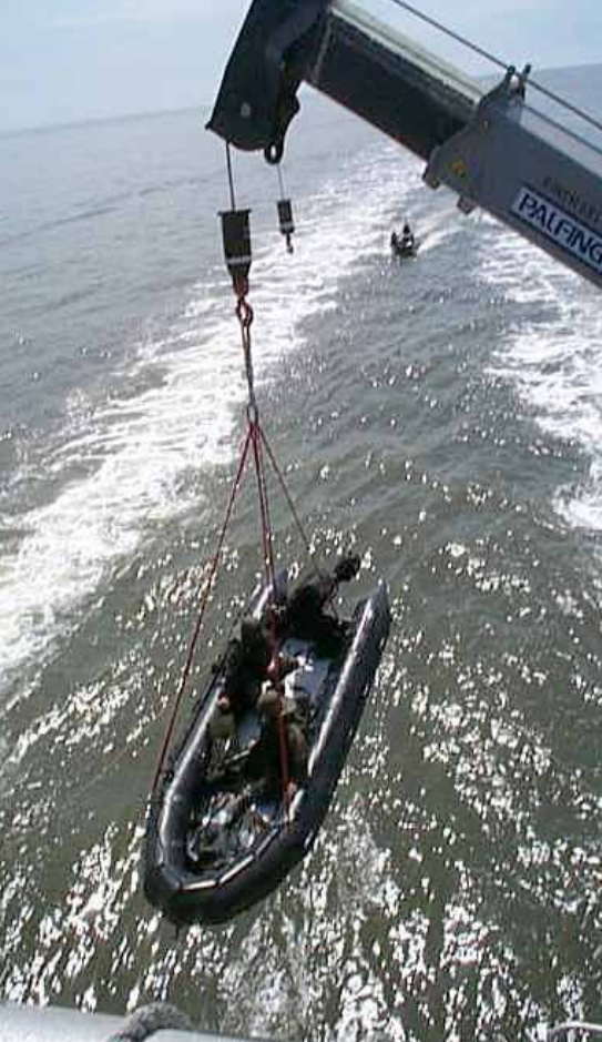
RHIB Launch Operations from Hull 061 HSV 2 Swift
