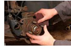
6. After removing the brake disc, clean the mating surface of the hub against which the old disc sat. This surface needs to be thoroughly clean to ensure the new disc sits flush and rotates true.
