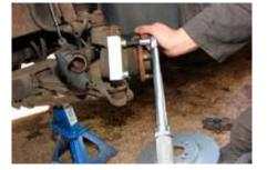
7. An anodised aluminium bracket needs to be fitted to make room for the larger discs. Two 10mm allen key headed bolts are supplied in the kit, which must be fitted with thread lock and tightened to 85Nm.
