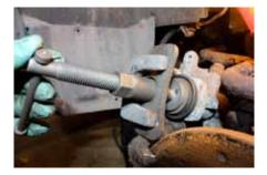
**12.** Fitting larger discs to the rear brakes is similar to the fronts. The only difference concerns retracting the caliper's piston, where a wind-back tool is required to turn the piston instead of pushing it in.
