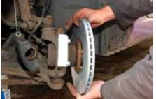
8. The new vented brake disc can now be fitted onto the hub. The original disc retaining screws are not required and the brake disc will remain secure once the wheel bolts have been fitted.
