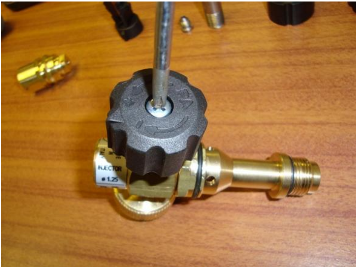
Step 9 Unscrew the black knob adjuster with a philips screwdriver
