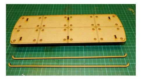
Glue the flatbed strakes to the Flatbed, using the engraved lines as a guide.
