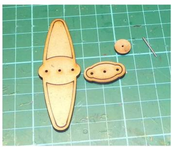
Glue the small connector onto the main coupling, using the pin, locate the circular plate into the centre.
