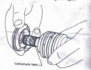
Install pinion assembly to pinion housing.
