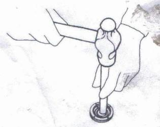
Install rear housing cover assembly to pinion.
